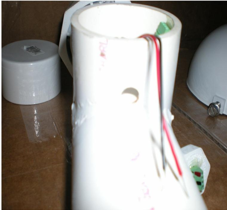
This view shows the penetration of the DS18B20 into the air stream in the pipe.
