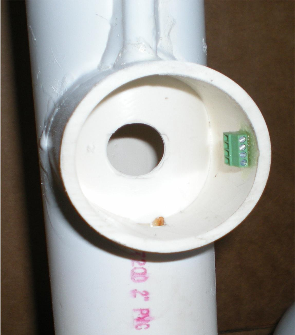
This view shows the cable hole in the bottom of the saddle, which also doubles to allow any water that might get in to weep out of the bottom of the junction box.
