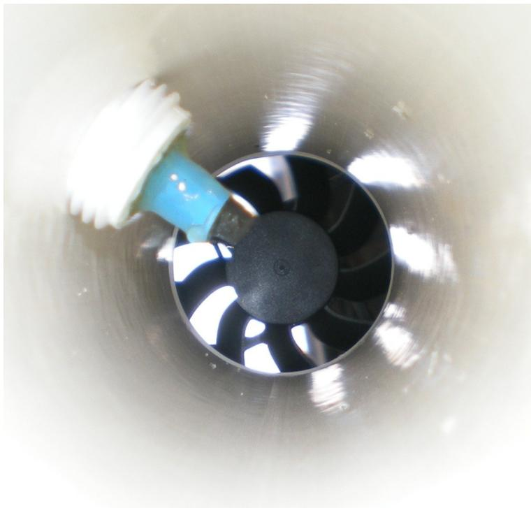
Here is an example all wired up. Green is 5V, Blue is 1-wire data, White/Blue is the ground for the 1-wire data and 5V. White/Brown is 12V, Brown is the 12V power return. The Orange pair and White/Green are unused. The 47 uF capacitor suppresses electrical noise from the fan.
