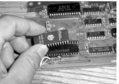
where pin 1 is. Installing the chip backwards will DESTROY THE CHIP and VOID THE WARRANTY! Draw a sketch if necessary!
