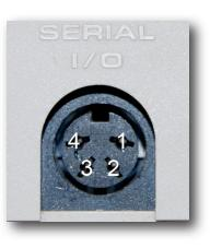
A 4 pin DIN connector shall be on one end of the cable which will mate to the jack on the back of the CoCo marked "Serial I/O". The other end of the cable shall be either a DB-9 or DB-25 female connector which will mate to an appropriate serial port on the Server.
