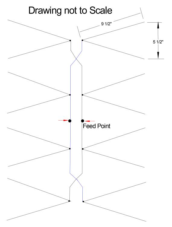
Most any metal will work for the elements. Try to use something near 1/8" diameter and make sure they are free of all coatings and oxidation where they connect to the phase line.
