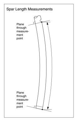
**H.3.2** Fittings, local curvature and local cut away, shall be ignored when measuring a **spar**.
