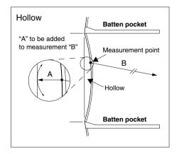
sail edge, the hollow shall be bridged by a straight line and the shortest distance from the measurement point to the straight line shall be measured. This distance shall be added to the measurement being taken.
