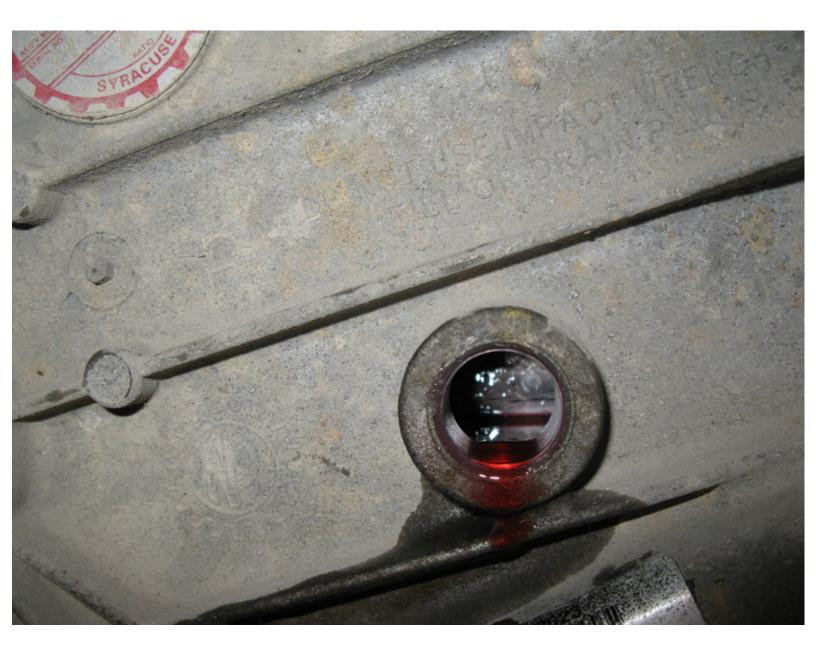
Finally, re-install the fill plug and you're done.
