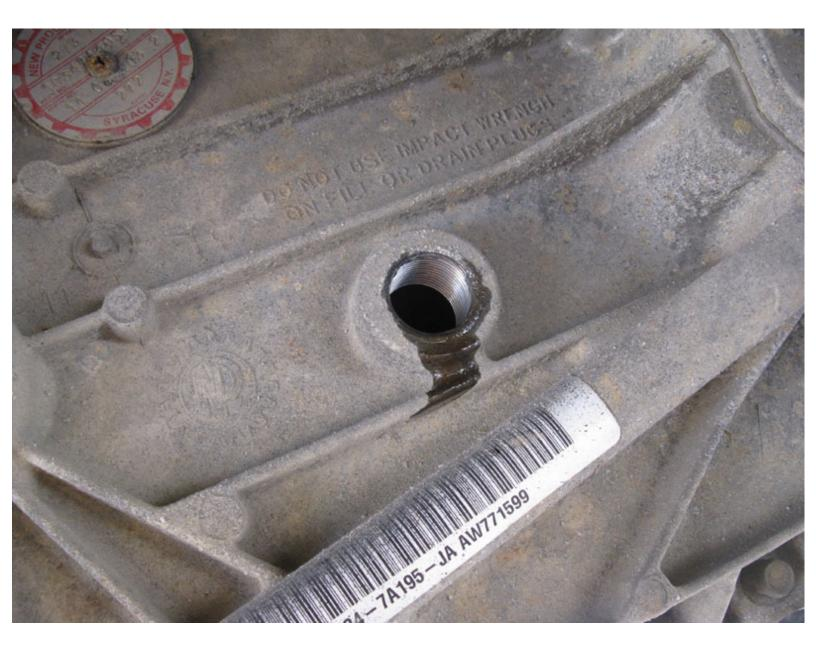
And then the drain plug. Allow the transfer case oil to fully drain.
