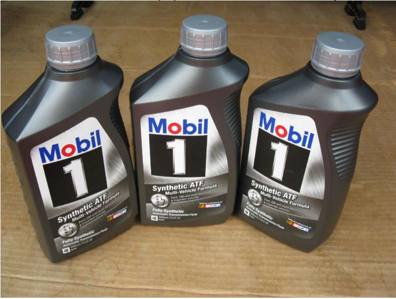
Here's the transmission fluid I used. Basically, any ATF that meets the MERCON or MERCON V specs will work.
