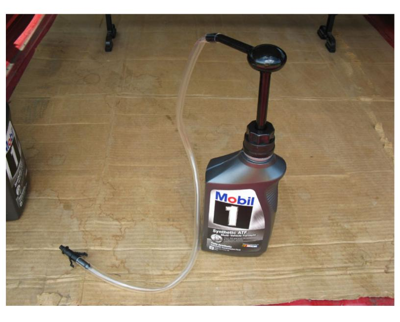
Insert the hose in to the fill hole and pump the new fluid in.
