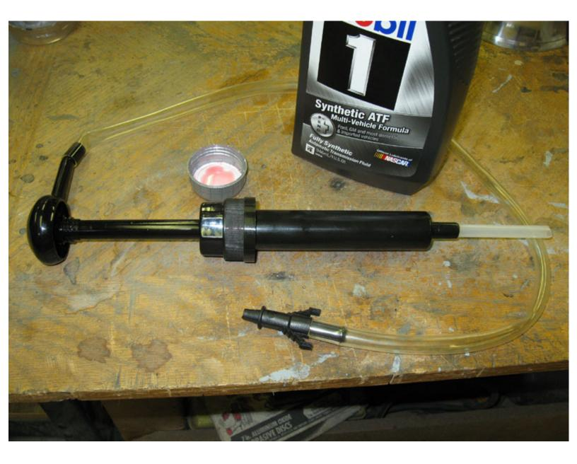
The adapter at the end of the hose is designed to hold it in various different sizes of holes.
