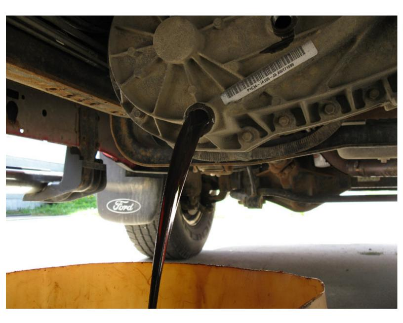
Once the t-case is drained, re-install the drain plug.
