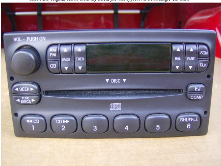
These generation Ford stereos are double-DIN units so the aftermarket options aren't so great. The most common option is to get a double DIN install kit which allows you to mount a single DIN unit at the top and use the remaining height of the double DIN space as a storage pocket. Here's an example of this kit from
