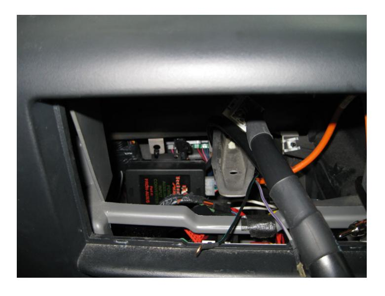
Next, connect the power and ground wires of the PIE adapter appropriately.
