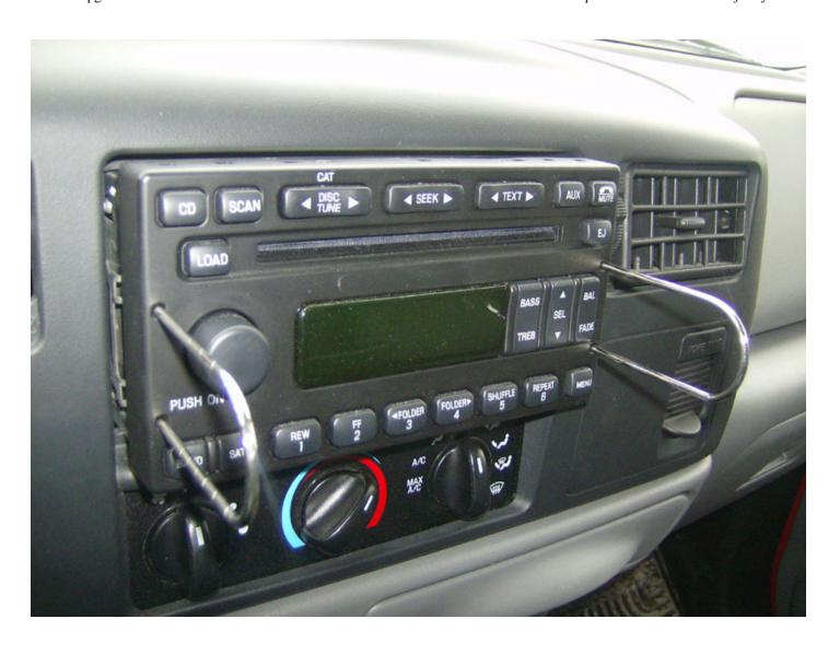
Then I plugged in the antenna cable and stereo harness in the new one, pushed it into the slot, and clipped it into place.
