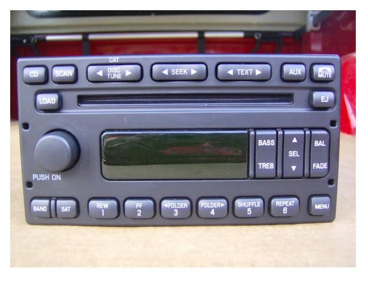
Not all auctions have good descriptions of what the unit really is. One way to easily distinguish a single-CD from a 6-disc changer is that the button to the left of the CD slot will have "LOAD" on it, on the CD6 models. On the single CD units, that button will just have "CD" on it. Some of the CD6 units actually have "CD6" written on the face somewhere, but not all of them.
