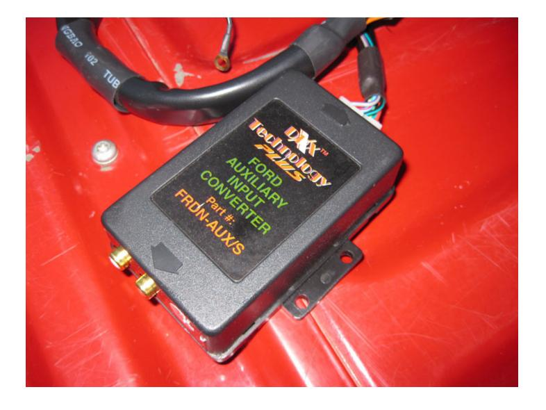
As you can see, this box has two RCA audio jacks on it for the input. A 3.5mm audio jack to RCA adapter cable would work well for this. However, I didn't want a cord dangling all the time, so I found the "Poly Planar IC-3.5M MP3 Adapter Cable" that has a 3.5mm panel mount audio jack. Then just connect the audio device, with a cable that has 3.5mm plugs on both ends, included with the kit.
