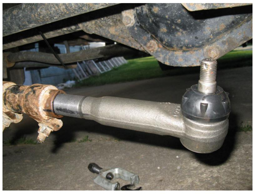
The new drag link was made slightly different than the original, so the measurement was not completely obvious even though I counted 22 turns. I ended up having to give it two more turns (tighter) from this point to get my steering wheel to be centered when driving down the road straight.
