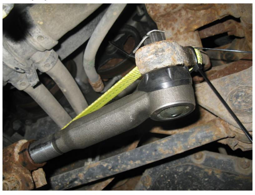
Finally, install the grease fitting, top it off with grease, and remove the straps and cables ties and you're done!
