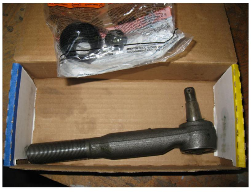
Here's the part in question, just a short part with an adjusting sleeve.
