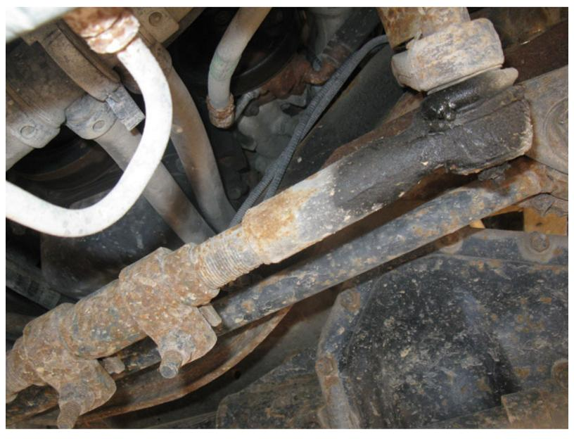
Its important to take a few measurements and count the number of turns it takes to remove it, so you can get the new one installed as close as possible on the first try.
