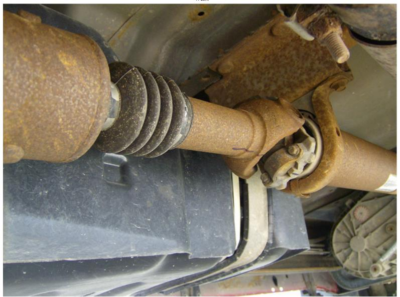
I spent some time making some unnecessary alignment marks. I've never had it apart before so I wasn't sure if there would be an opportunity to get the splines misaligned. Turns out you cannot connect the slip yoke incorrectly because there is one "double spline" allowing only one way to connect it. You only have to remove the front clamp (red arrow) to get it apart.
