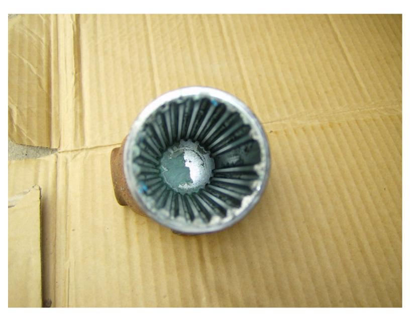
I applied plenty of grease to the splines. Way too much actually as most of it got pushed out when I reconnected the slip yoke assembly. Oh well, I'll know to use less next time!
