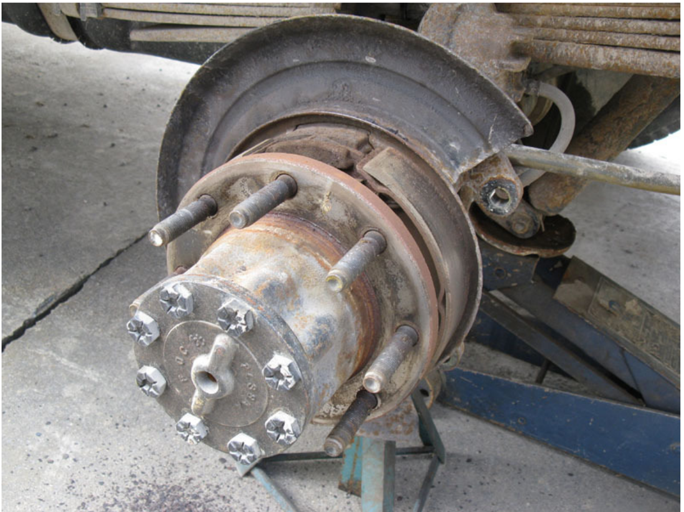
Here's the wear on the rotor.
