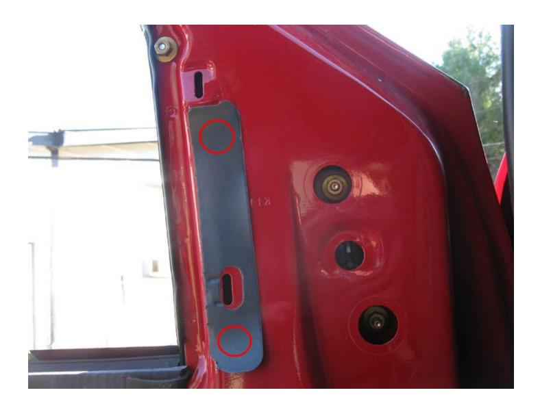
Now with the mirror removed, the hole for the wiring can be drilled. You might notice that the mounting location of the LED module doesn't match the final location shown at the end of this writeup. As expected, I had to tweak the location a bit. I originally thought it would help to have them angled rearward a bit but it turned out that was a bad idea. I adjusted them to pretty much just point straight down.
