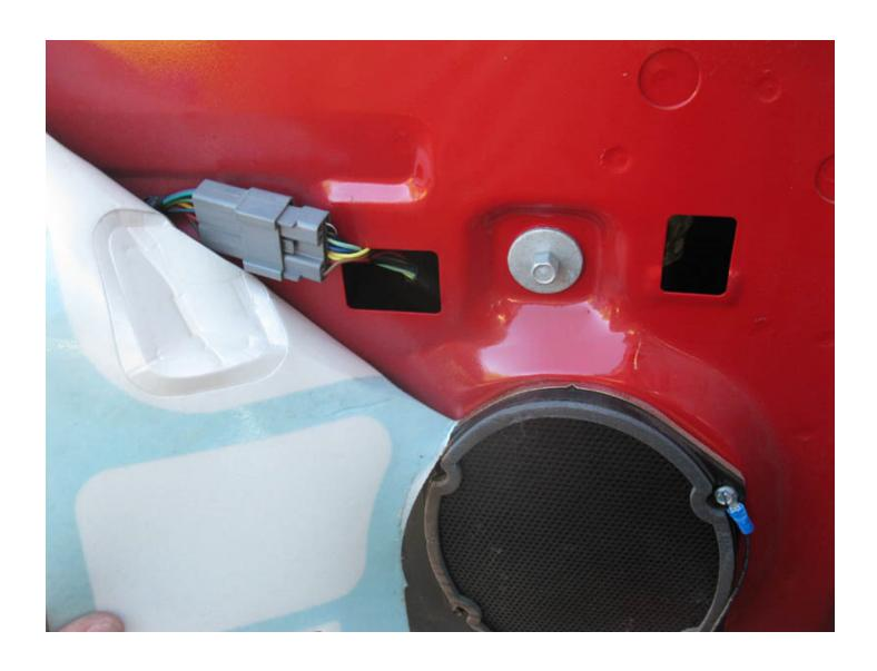
Then remove the two large rubber plugs. You can leave the middle plug in place.
