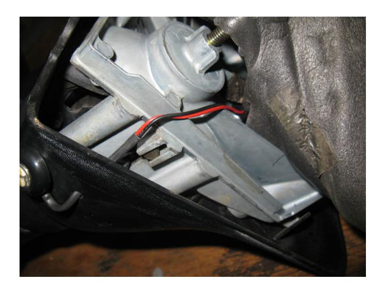
I also drilled a small hole in the mirror structure to allow the wiring to pass through. Otherwise it would've been pinched between the mirror and the truck body. Again, a little heat shrink was added for protection.
