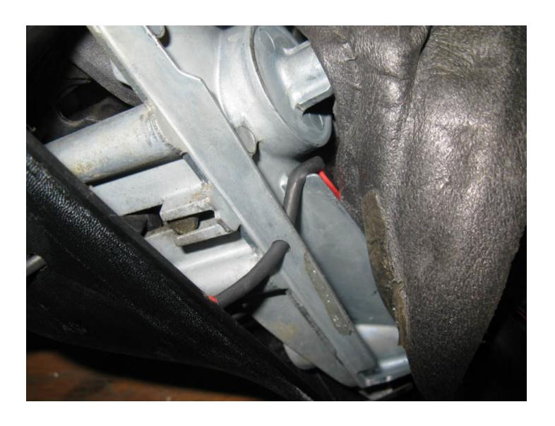
Next, reinstall the mirror and rubber plugs, then fish the wiring harness back up out of the door and reconnect it. The wires that came on the LED module were long enough to get to this point, but not long enough to connect to where they needed to go. So, I soldered and heat shrinked a couple short wires to them to finish them off
