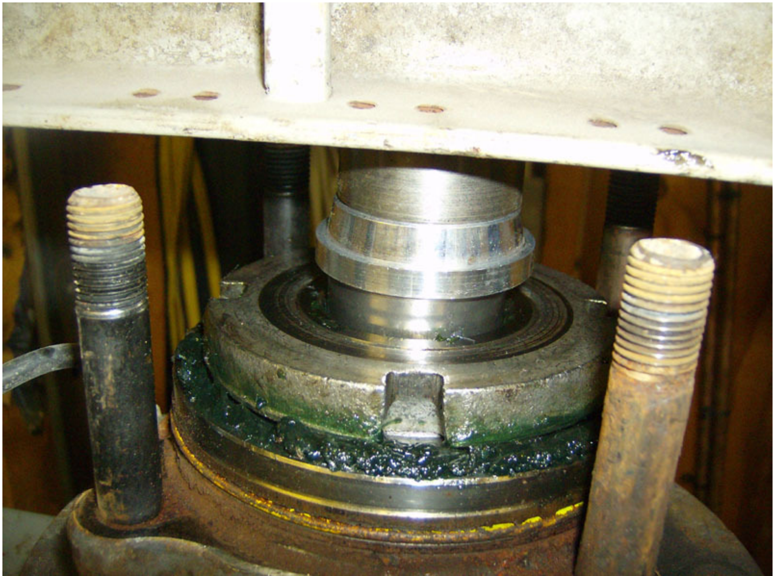
There you have it, new needle bearing installed.
