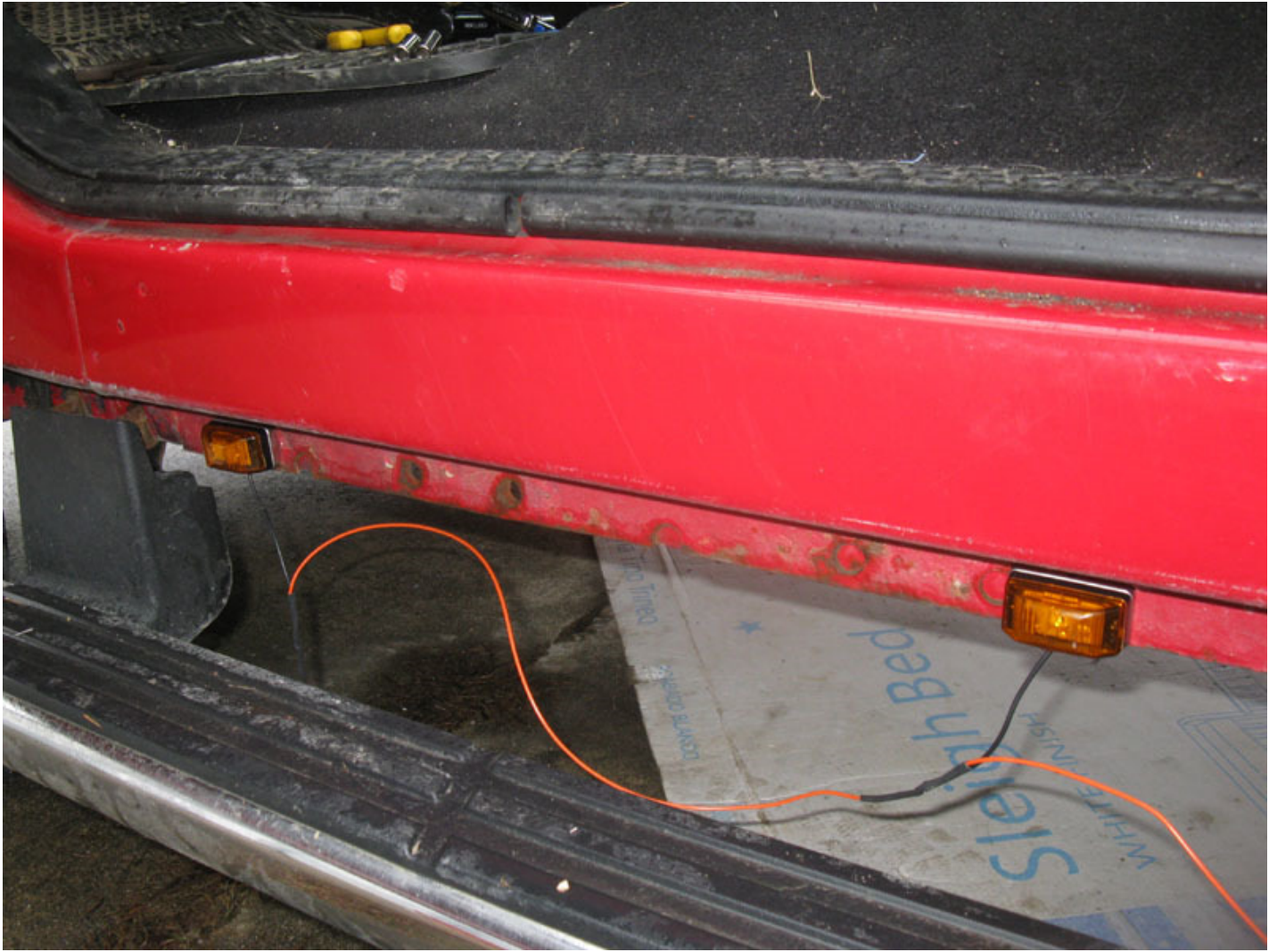
Here's a shot of the wiring from the backside.
