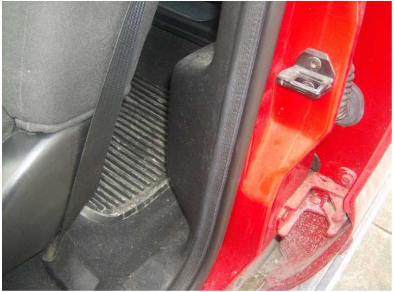
I first removed the lower trim piece along the bottom of the door and peeled the weather stripping back.
