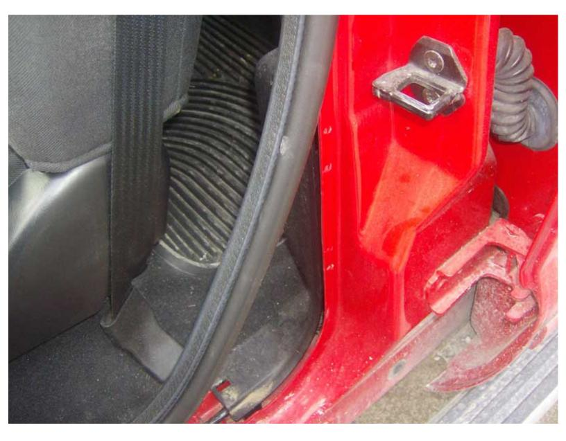
Next I removed the trim and peeled back the weatherstrip for the rear door.
