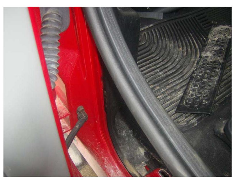
Next I pulled the center trim piece away from the door post enough to get my hand in there for the install. It pops out by pulling it toward the center of the cab. Don't forget to pull out this clip hiding at the bottom of this trim piece.
