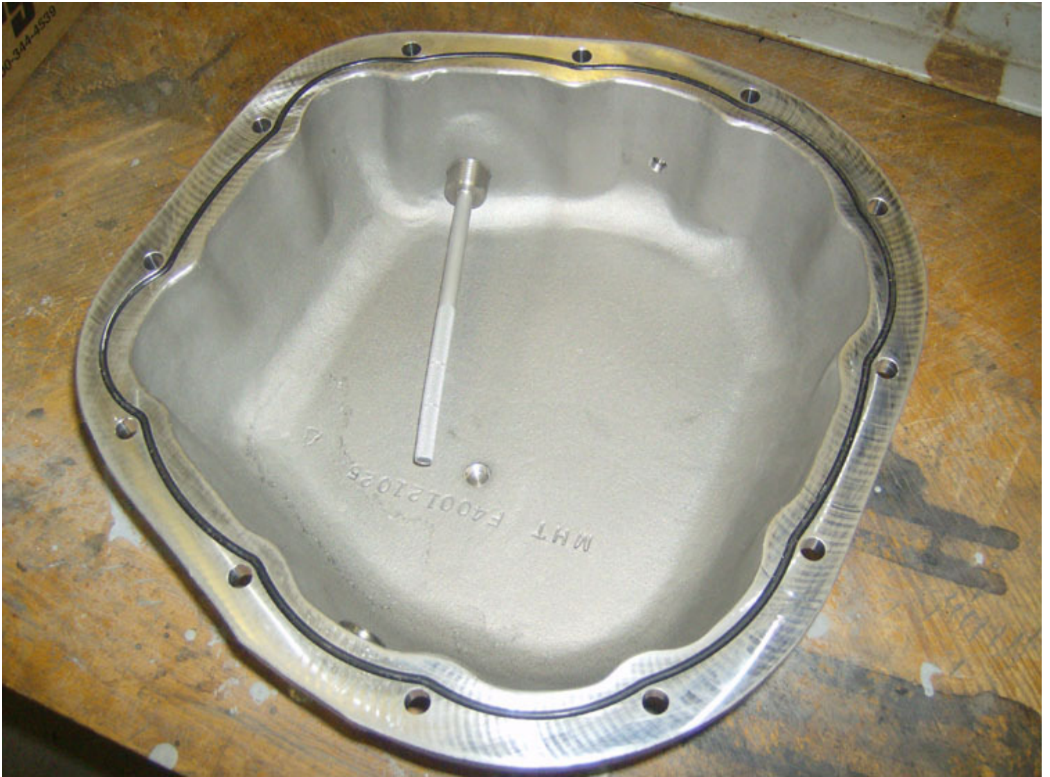
Here's a shot of the dipstick (left) and temperature sender port.
