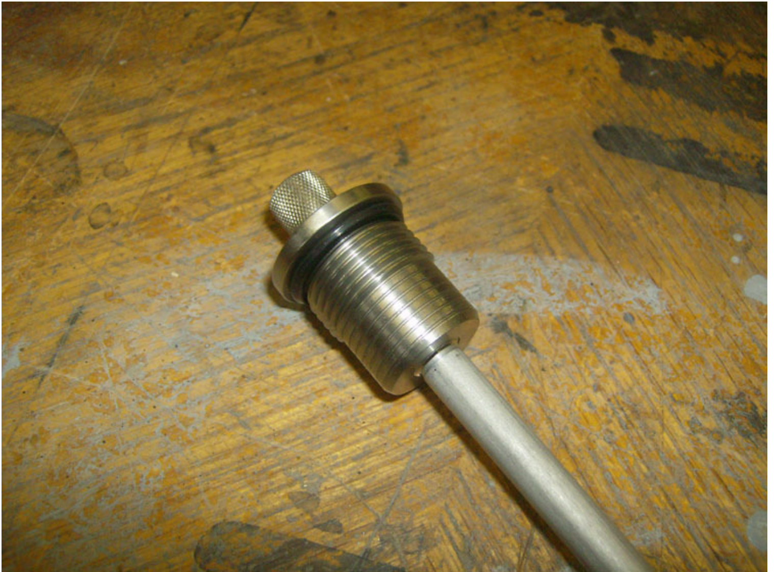
Drain plug removed
