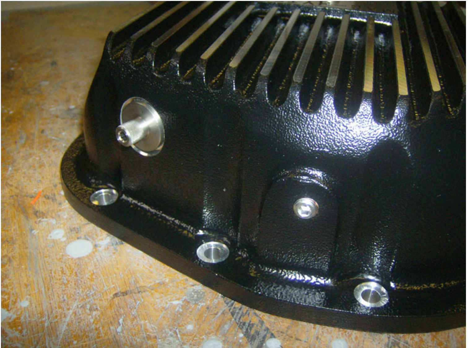
Here's a pic of the drain plug on the bottom.
