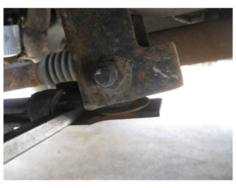
Here's the pad. It is very thin and was VERY dirty/rusty before I cleaned it up. I suspect some of the squeaks were caused by the metal-on-rusty pad motion.
