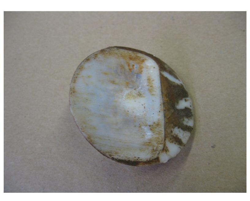
Since I didn't have new pads, I decided to implement a temporary fix by cutting a "donut" out of some 1/8" thick teflon material that I had laying around. I'll use this to beef up the original pad until I can find some new ones.
