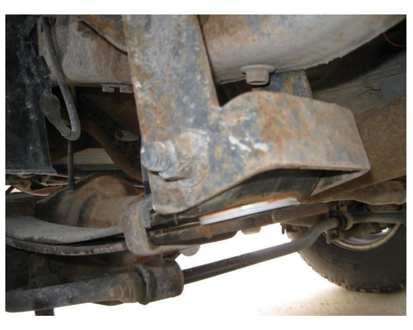
Now for the "main squeaker" that I found. This is the pad on the rear of the passenger side front spring. Definite metal-on-metal contact in this case!
