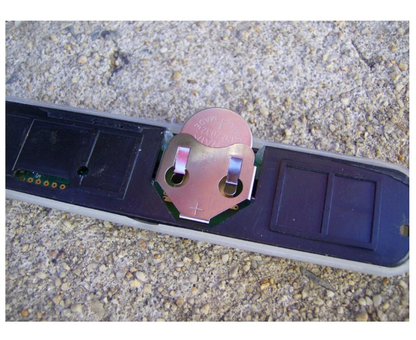
After installing the new battery, just insert the "membrane" back into the plastic housing, and snap it all back together.
