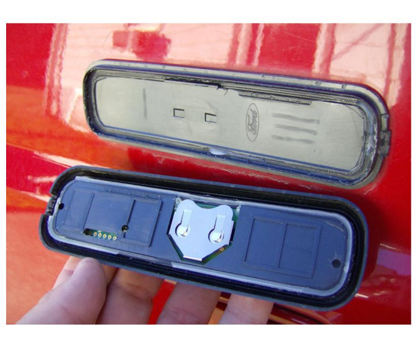
Next I removed the "membrane" part from the plastic housing to access the battery easier.
