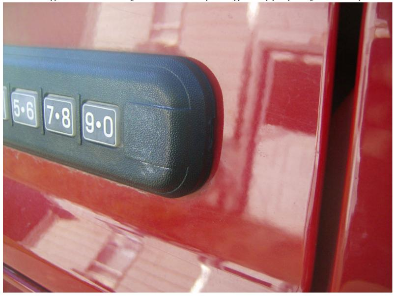
Use the biggest flat screwdriver that you have (that fits in this notch) and pry it apart. This unit snaps together pretty tight so it does take some work to get it apart without breaking it, and without scratching your paint.
