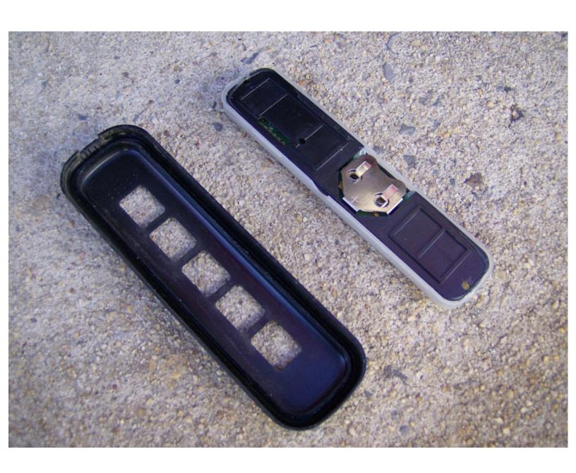
I think these keypads are supposed to use a 3V battery # 2335. I didn't have one handy but I did have a 3V #2032 which was the same physical size so I used it. It works fine. Time will tell how long it lasts.
