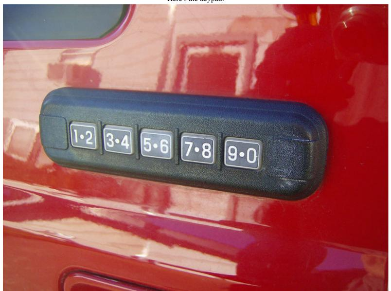
The keypad has a notch on the right side which is where you're supposed to pry it apart to get to the battery.
