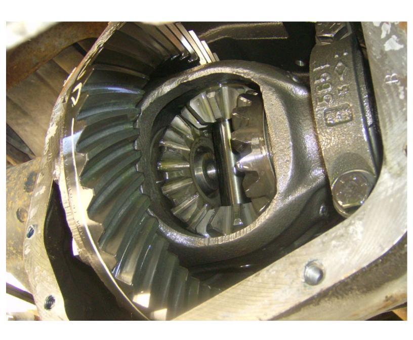
Next, place a rag around the gears to keep the gunk out of them while cleaning up the gasket surface.
