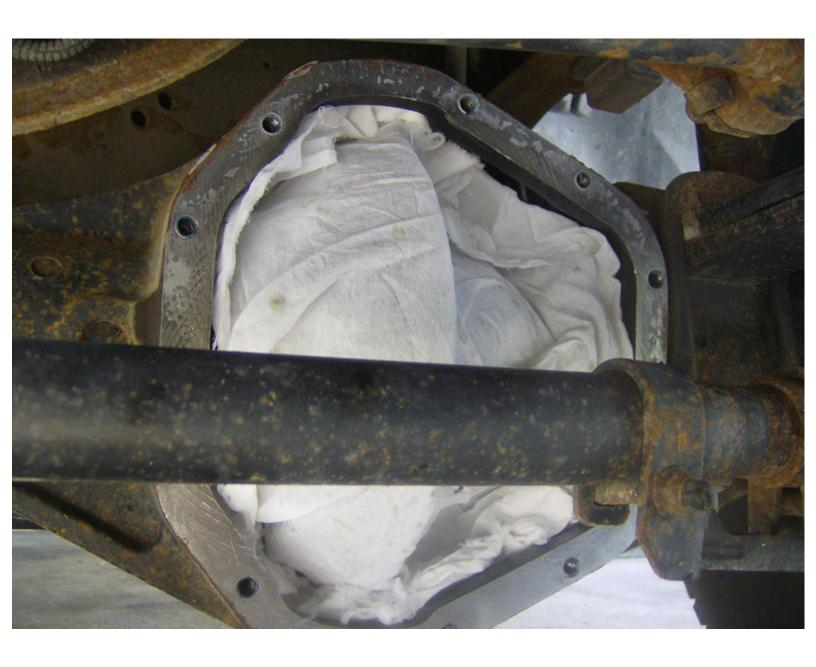
I cleaned up the gasket surface using the same steps I did on the cover -- scraper, scotchbrite pad, rags, lacquer thinner.
