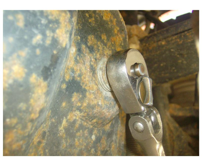
Remove the front differential cover by removing the bolts. Nine of them are 9/16" hex head bolts and one is a socket head cap screw (with a washer) that requires a 5/16" allen wrench. I left the two top bolts in place to hold the cover while the bulk of the oil drained out.
