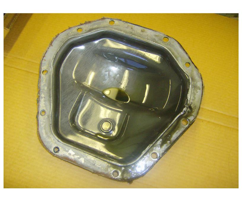
I cleaned the gasket surface with the scraper tool, then cleaned the area with a scotchbrite pad, and then did the final cleanup with some rags and lacquer thinner.
