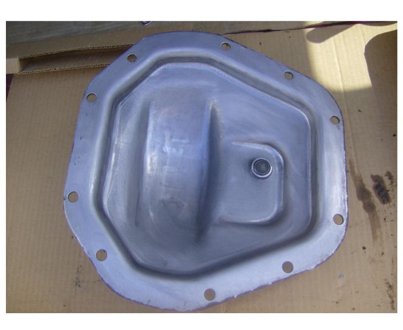
Its pretty typical for the cover to have rust on it which could eventually lead to problems. I spent a few minutes with the 4" angle grinder cleaning up the worst of it. Then hit it with some primer and paint.
