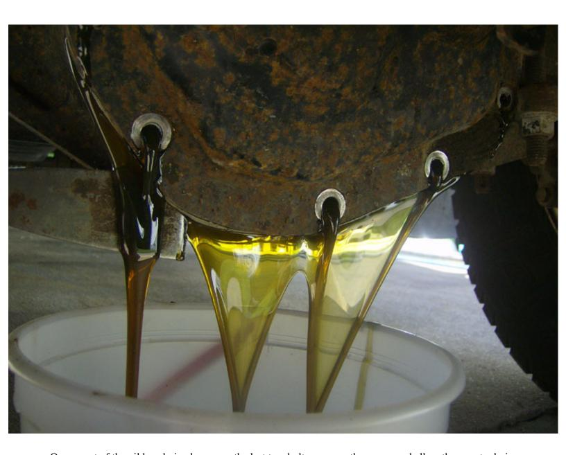
Once most of the oil has drained, remove the last two bolts, remove the cover, and allow the case to drain.
