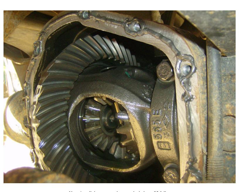
Next, install the cover and torque the bolts to 35 ft lbs.
