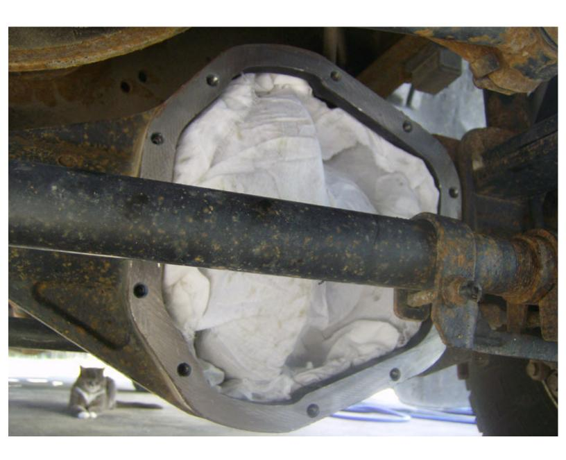
Now that the axle housing and cover are both clean and ready for reassembly, the next step is to apply the RTV gasket sealer. I put about 1/4" bead around the perimeter, circling the holes. Let the RTV skin over for about 20 minutes.
