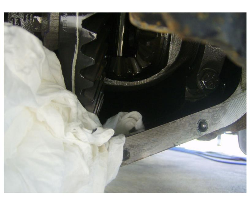
Inspect the gears to make sure there are no chipped teeth, cracks, or weird looking wear patterns.
