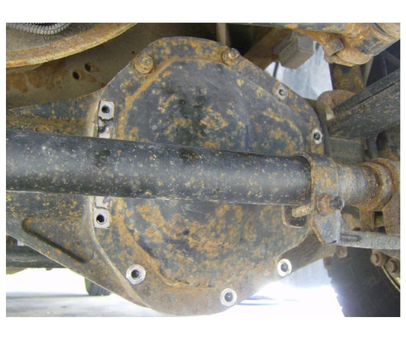
Use the scraper tool to break the seal and let the oil drain.
