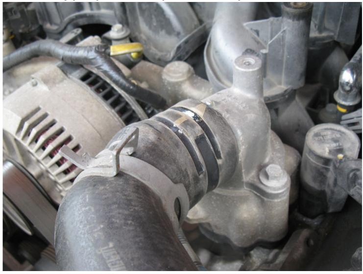
Use a large pair of pliers to release and pull back the hose clamp, and disconnect the hose.
