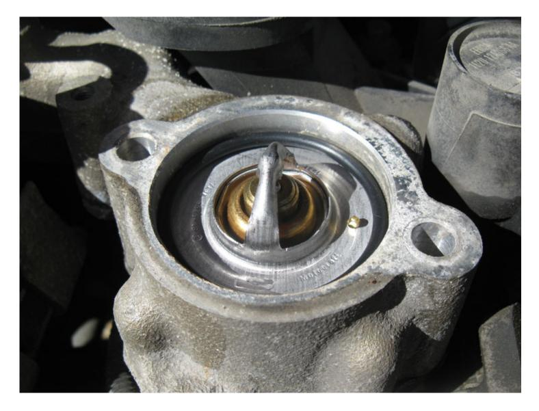
After re-installing the thermostat housing, the hose, and the hose clamp, I refilled the reservoir with a little over three gallons of antifreeze.
