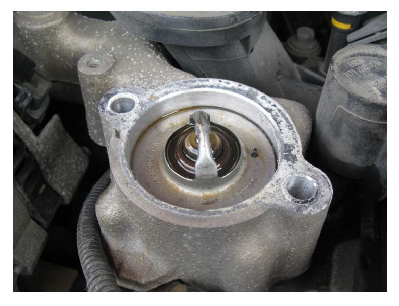
Remove the thermostat and re-install the thermostat housing, without the o-ring
