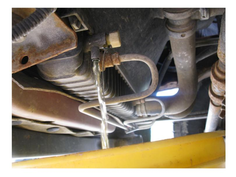
Then tighten the draincock and refill the reservoir with distilled water, it took about three gallons on mine. Also, pour in the two bottles of Super Flush. Run the engine for about 15 minutes with the cab heater turned on high.
