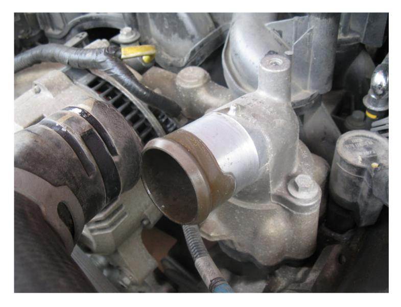
Remove the two bolts holding the thermostat housing in place
