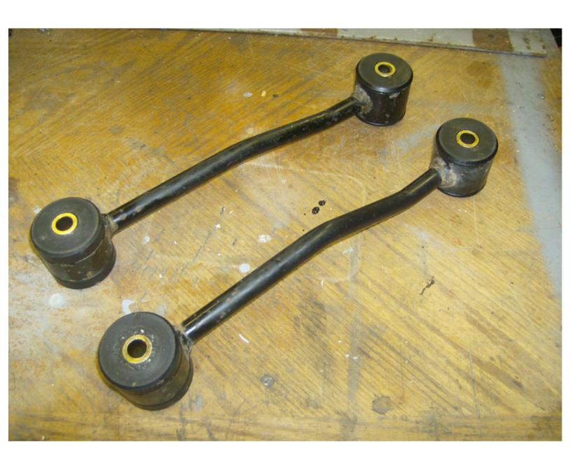
Now you can remove the old bushings from the sway bar and install the new ones in the same location. Also remember to apply the grease to the inside of these bushings where they contact the sway bar.
