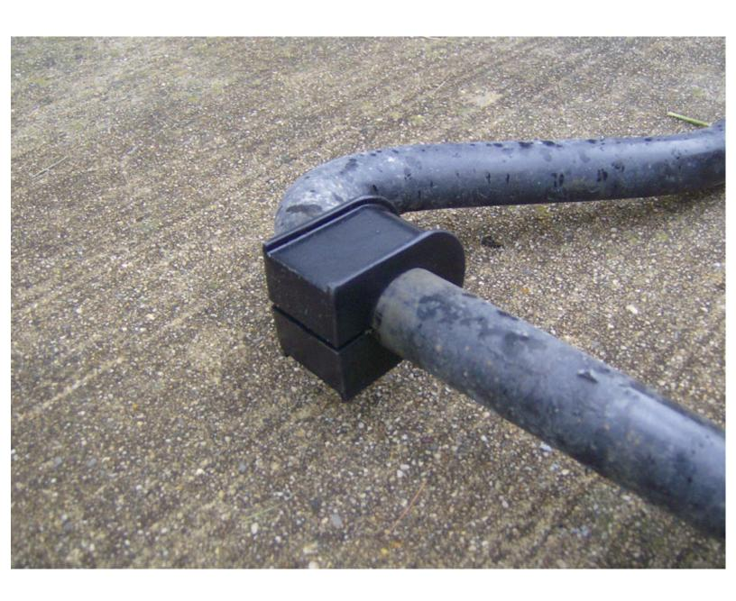
Now it is time to reinstall everything. I first reinstalled the sway bar to the axle. Again, I put a layer of grease on the outside of the bushings, where the U-shaped metal straps contact the bushing. I reinstalled the four nuts and left them loose.
