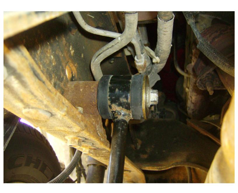
Next, on the passenger's side, I removed the bolt that goes through the end link and frame. You cannot remove the end link at this point because the bolt hits on the exhaust pipe. So, you must remove two bolts from the bottom side of the frame, that connect up into the spacer block. Now you can remove the passenger side end link.
