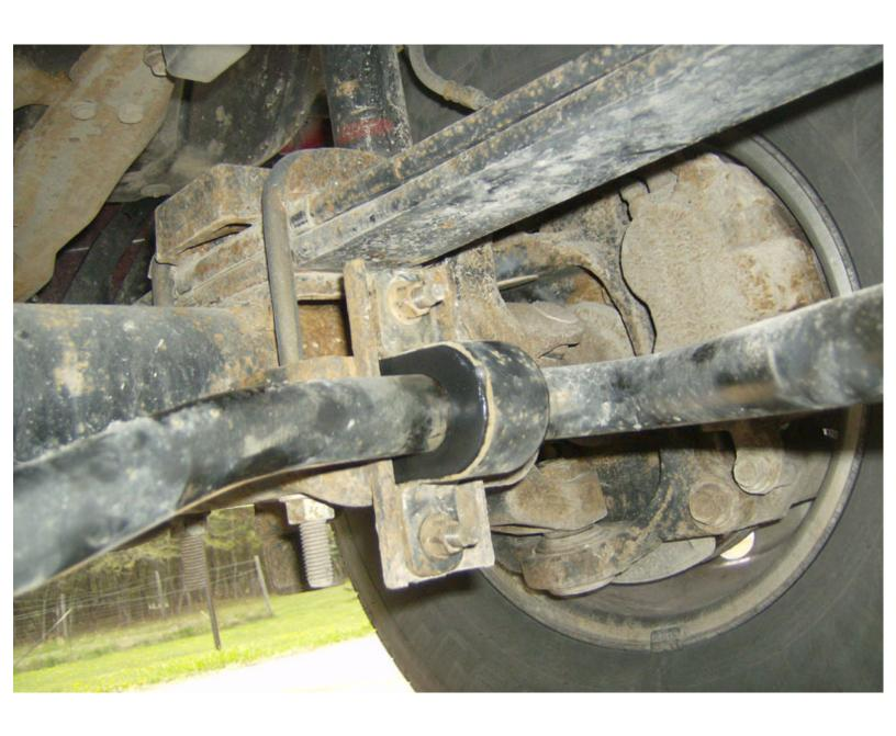
Next I removed the driver's side end link by removing the bolt that goes through the end link, spacer block, and frame.
