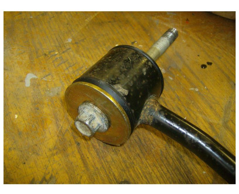
Next I installed the two bolts back through the bottom of the frame, into the block, and left them loose. Then, I tightened the bolt that goes through the end link, block, and frame. Then tightened the two bolts that go up into the block.
