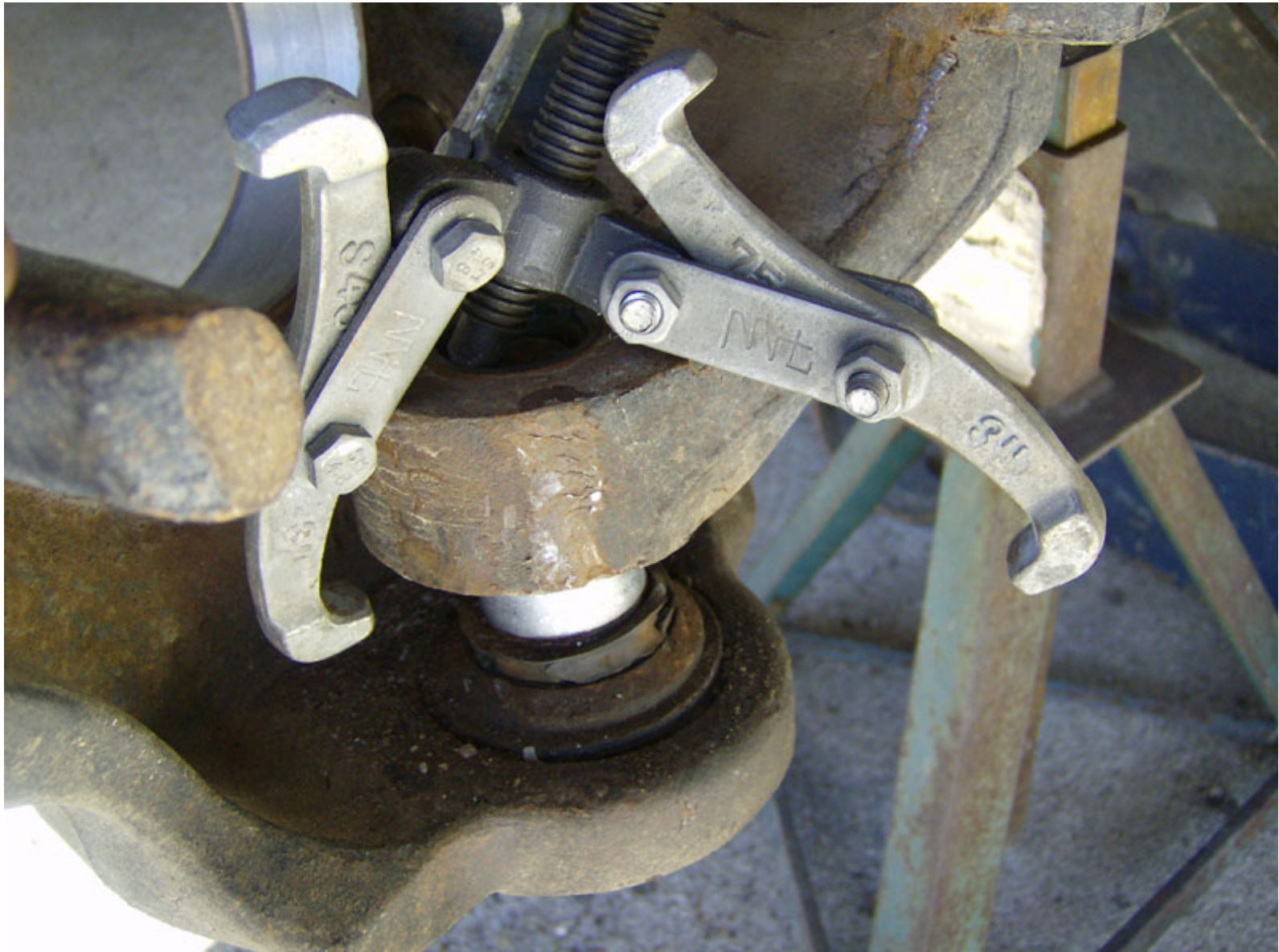
Once both ball joints are free, remove the nut from the top one, and remove the knuckle.
