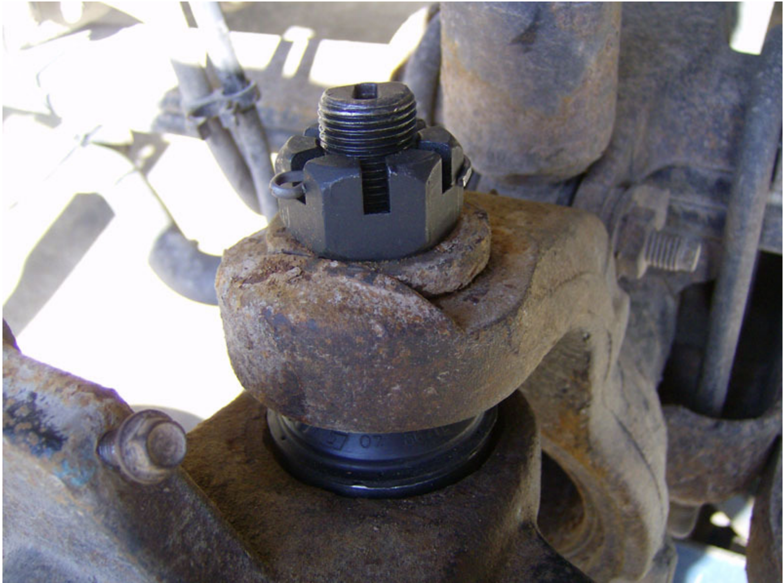
Here's the knuckle fully installed.
