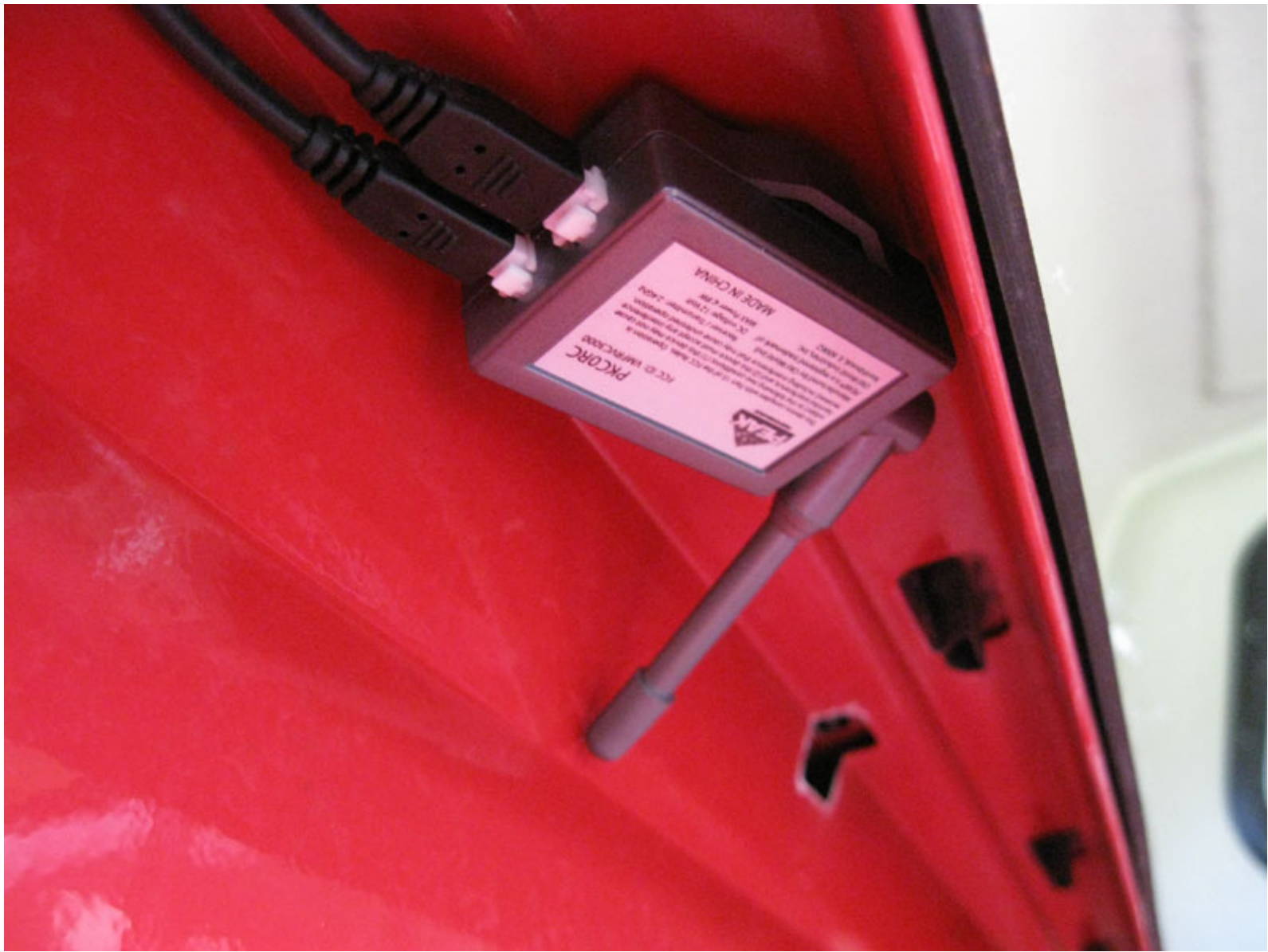
Here's the camera installed on the license plate. The kit comes with wedges which I had to use to angle the camera down to get a better view.
