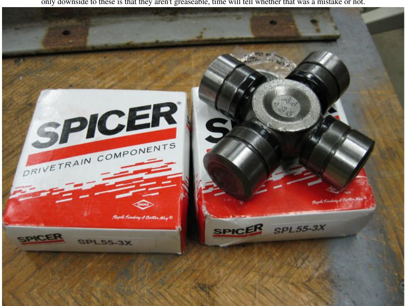
The process of replacing axle u-joints is fairly straight forward, although they can be a real pain sometimes. I used my press to remove & install them but before that I used a bench vice in place of the press. Same principle, just a little more difficult. Its also very useful to have another person to help with this process, particularly on the passenger side axle that is quite long and heavy.
