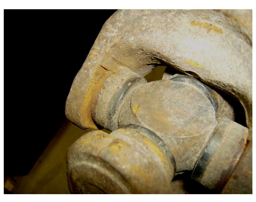
Spray penetrating oil on the u-joint cap areas and let it sit for 10-15 minutes. Then set the axle up on the press as shown below. Use a collar to support the bottom that is open in the middle to allow the u-joint cap to be pressed down. Use a small collar on the top to drive the u-joint down, without contacting the yoke, on the topside.
