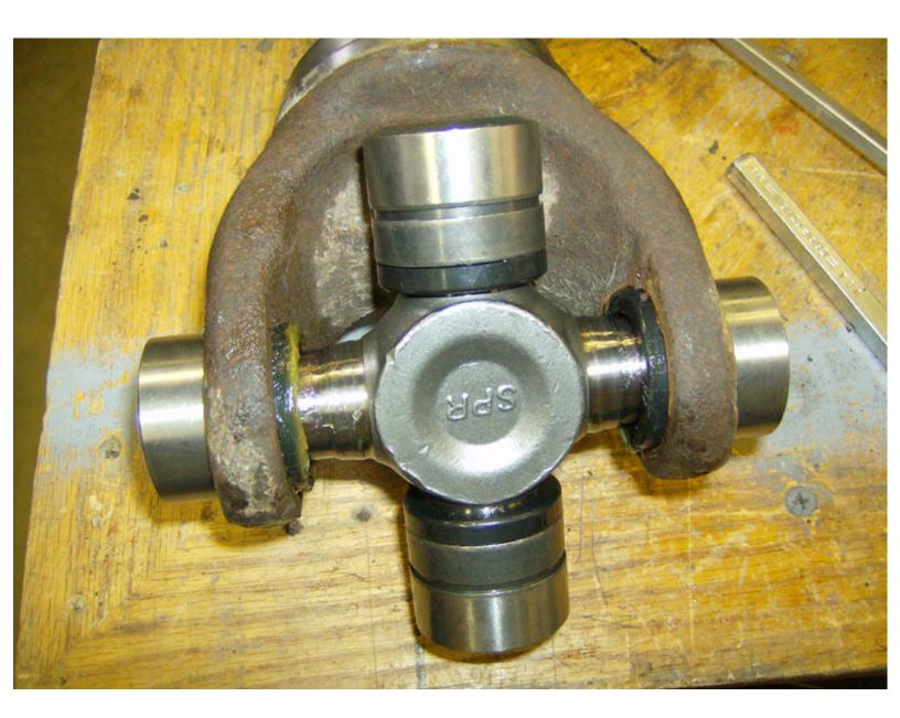
Use the press to install the new caps until the C-clips can be installed.
