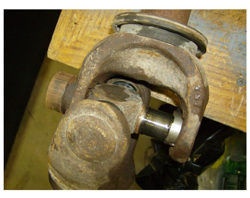
Here's where the u-joint used to be.
