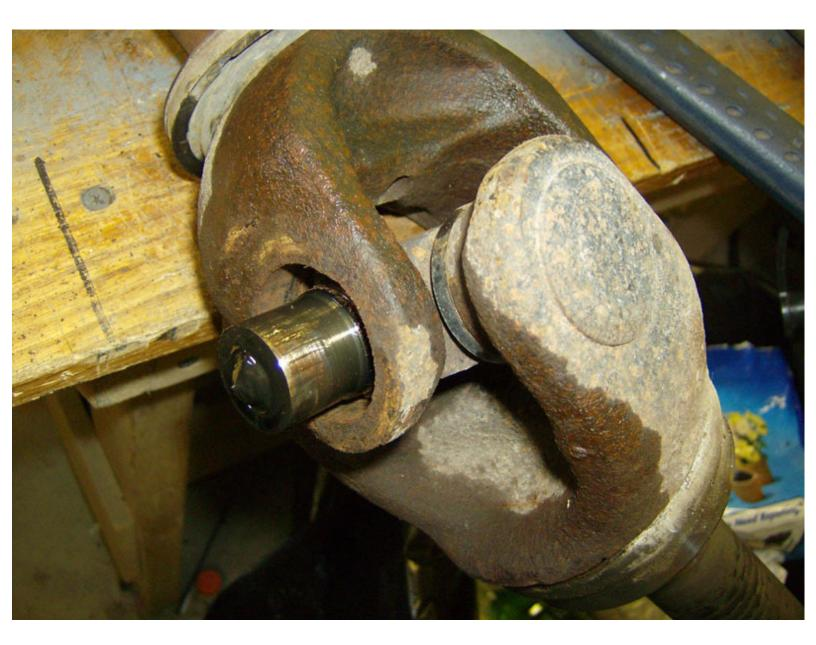
Go back to the press and set it up opposite of the first press operation and drive the other cap out of the opposite side of the yoke. Pull the cap off of the u-joint and then you can remove it from the yoke.
