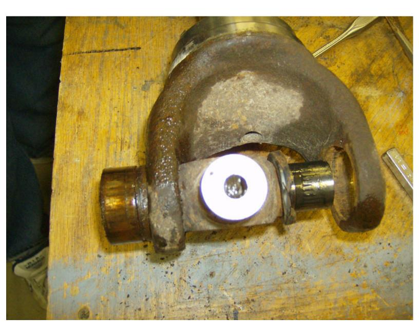
Now its time for the new u-joint. After cleaning up the cap surfaces and the C-clip areas, remove the caps from one axis of the u-joint, place it in the yoke, and start the caps into their holes.
