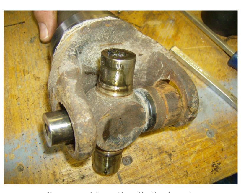
Now you can remove the last cap, and the rest of the u-joint can be removed.
