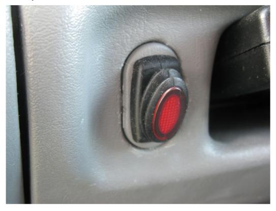
This switch is smaller, so I had to mount it in the original plug for the oval hole in the dash.
