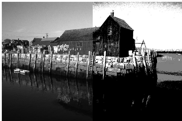
motif1_g_comp The Green channel of the original image as a grayscale image. The left half has 256 levels (8-bits) while the right half has 8 levels (3-bits).
