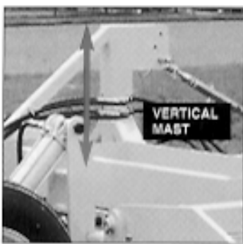
Make sure the mast is completely vertical for maximum control of the tine angle.
