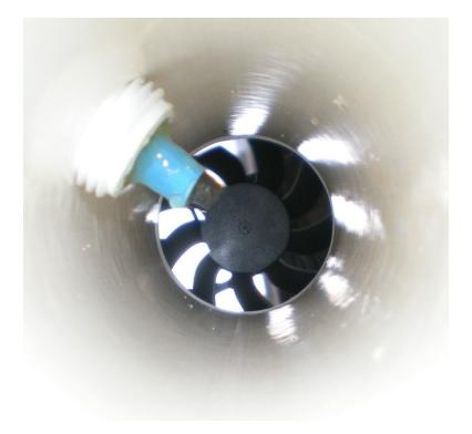
Here is an example all wired up. Green is 5V, Blue is 1-wire data, White/Blue is the ground for the 1-wire data and 5V. White/Brown is 12V, Brown is the 12V power return. The Orange pair and White/Green are unused. The 47 uF capacitor suppresses electrical noise from the fan.
