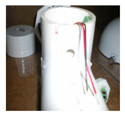
This view shows the penetration of the DS18B20 into the air stream in the pipe.
