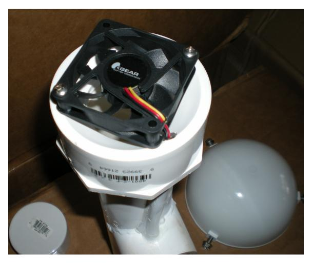
Another view of the saddle showing the Phoenix connector used to connect the fan wires and capacitor. Note that the tapped hole for the temperature sensor assembly is offset to one side so that you can get a 1-1/8" deep socket over the PVC plug without hitting the Phoenix connector glued to the side of the junction box.
